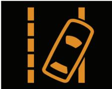
In road-transport terminology, a lane departure warning system is a mechanism designed to warn the driver when the vehicle begins to move out of its lane (unless a turn signal is on in that direction) on freeways and arterial roads. These systems are designed to minimize accidents by addressing the main causes of collisions: driver error, distractions and drowsiness.
